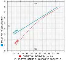
These pumps are advised for the transfer of low-high viscosity oil and similar fluids for medium-long distances. The delivery capacity of a pump varies according to particular applications and combinations. The operating pressure may vary between a minimum of 3 bar and a maximum of 8 bar.
