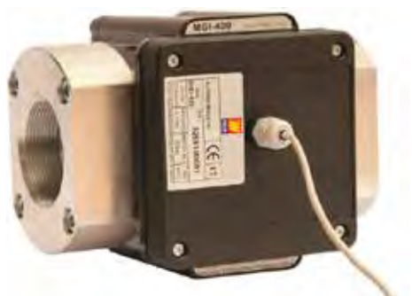
Art. 092-5170-400 Mechanical pulsed flow meter MGI-400 min-max flow rate 15-400 l/min nr. 5,5 pulses/liter
