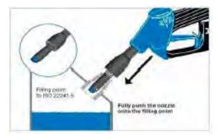
Most light vehicles <3,5 t allow a trouble-free filling of the AdBlue® tanks with a flow rate of not more than 5 l/min. The nozzle should be adjusted to this value for daily operation.
